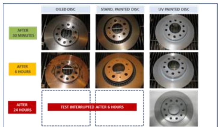
Moisture resistance test
